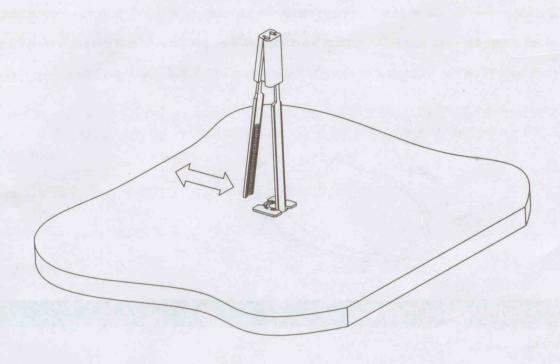
Align the seat fixing holes over the plastic collar and fix with the bolts provided.
