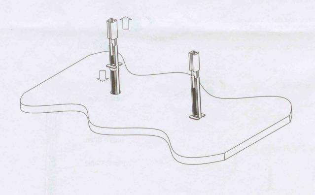
Snap the toggle strap off, by holding it at the plastic collar and moving it from side to side. Ensure the straps snaps off flush to the plastic collar.
